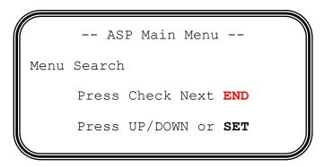
2) Press the END button. The error beeping will end and the screen will show the following screen: Press the SET button. (The Main Shaft will rotate to the "o" Degree Mark or the Fixed Position automatically.
